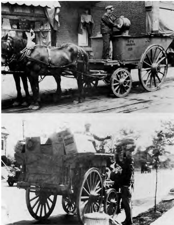
Figure 1-1 A typical horse-drawn solid waste collection vehicle, used well into the 1920s in many U.S. cities. (Courtesy NCRR)
