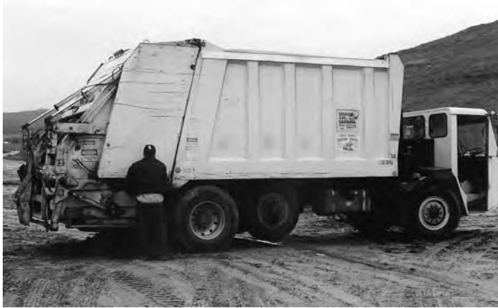
Figure 3-2 A rear-loading packer truck for collecting residential solid waste. (Courtesy William A. Worrell)
