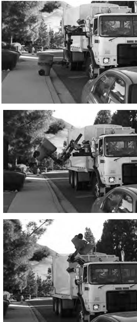
Figure 3-7 Collection with vehicles equipped with “can snatchers.” (Courtesy Peter Cron)
