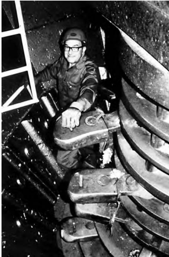
Figure 5-10 Inside a vertical hammermill shredder. (Courtesy William A. Worrell)
