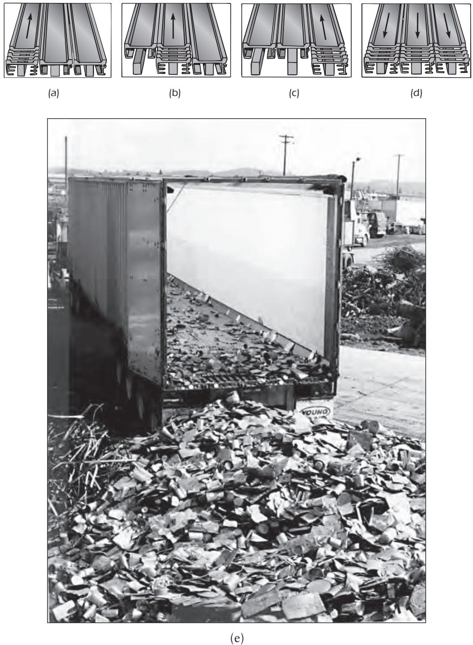
Figure 5-4 Truck equipped with moving floor. (a) The first slat group slips under the load to the rear of the load. (b) The second slat group slips under the load. (c) The third slat group slips under the load. (d) All slat groups and the load advance forward together. (e) A truck equipped with a walking floor has just emptied its contents. (Courtesy KEITH Mfg. Co.)
