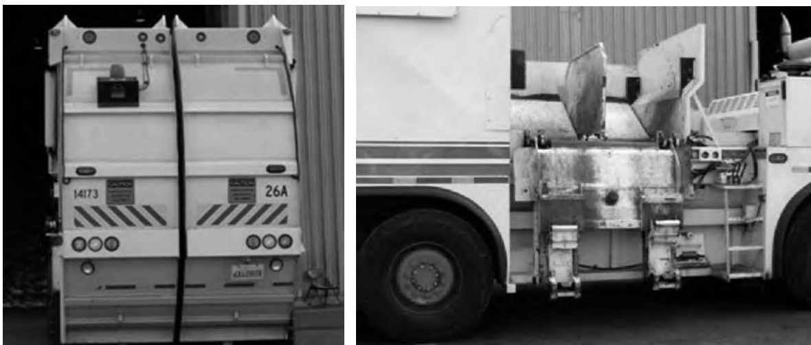
Figure 3-18 Dual-compartment packer truck with dual tippers. (Courtesy William A. Worrell)
