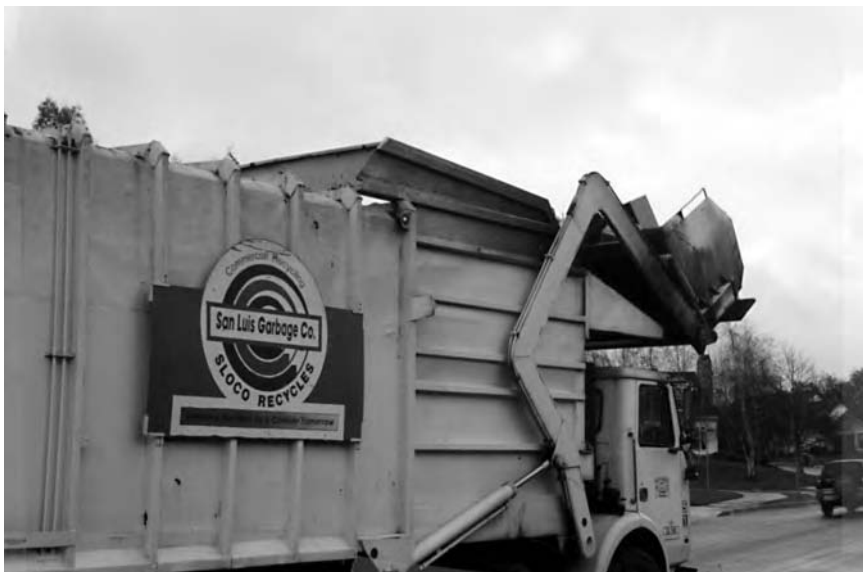
Figure 3-19 Multicompartment truck for collecting separated recyclable materials. (Courtesy William A. Worrell)
