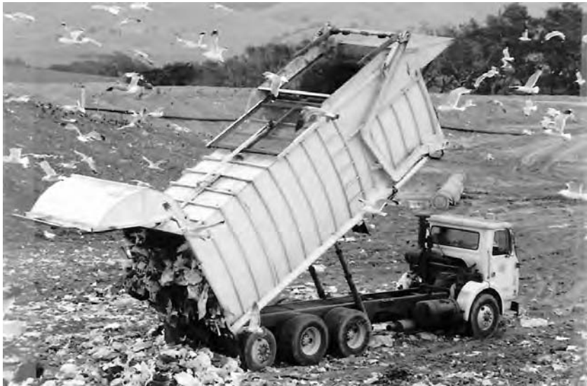
Figure 3-14 Dumpster collection truck being emptied at a landfill. (Courtesy P. Aarne Vesilind)
