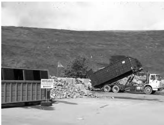
Figure 3-14 Dumpster collection truck being emptied at a landfill. (Courtesy P. Aarne Vesilind)
